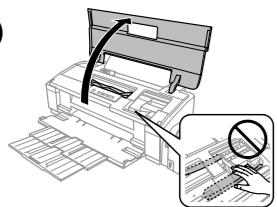
Open the printer cover and remove all of the paper inside, including any torn pieces.
